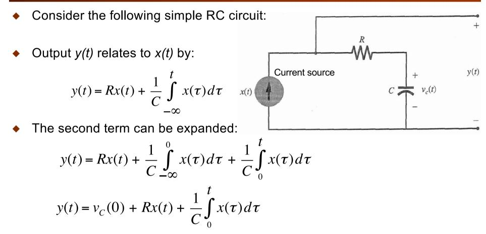
This is a single-input, single-output (SISO) system. In general, a system can be multiple-input, multiple-output (MIMO).
